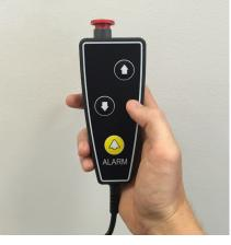
**Handset on spiral cable** on the platform allows to comfortably control the platform while sitting in the wheel-chair or on the folding seat
